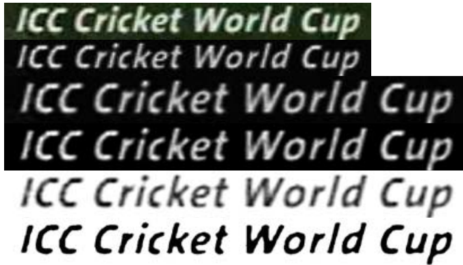
1. ORIGINAL IMAGE 2. GRAYSCALE IMAGE 3. INTERPOLATION 4. QUANTIZATION 5. INVERT 6. THRESHOLDING 7. OCR.
