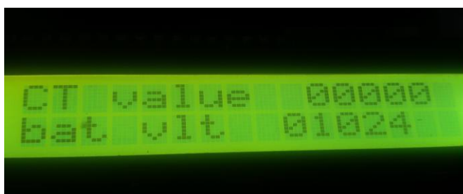
Fig. 6 Display of current present in load and battery voltage
