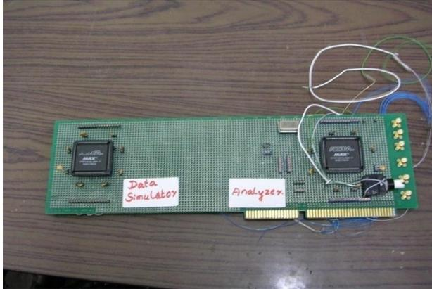
Fig 2 Data simulator and frame sync detector
