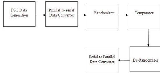
Fig:1.,signal flow diagram for Data Simulator and FSC detector
