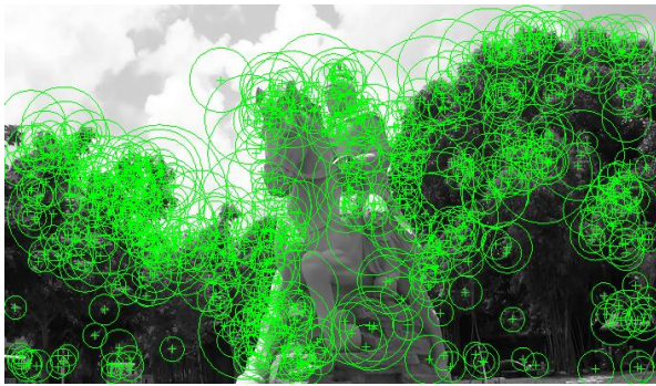
Fig. 2 Feature extraction using SURF algorithm
