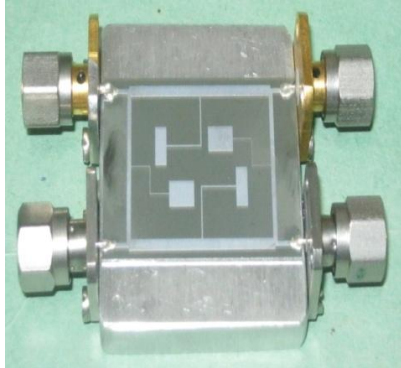
Figure 11. Photograph of the fabricated branch-line .
