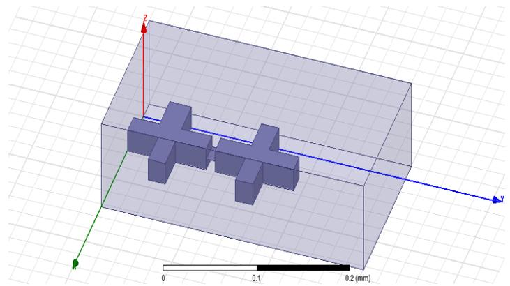
Fig. 3. HFSS layout for the Cubodical nano rod.
