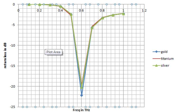
Fig. 7. Return loss of Au, Ag, Ti Nanorods.
