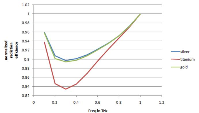
Fig. 8. Normalized Radiation Efficiency of Au, Ag, Ti Nanorods
