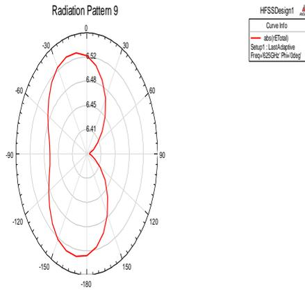
Fig. 5. Radiation pattern of the cubodical gold nano rod
