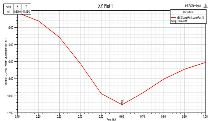
Fig. 4. Return loss of the cubodical gold nano rod
