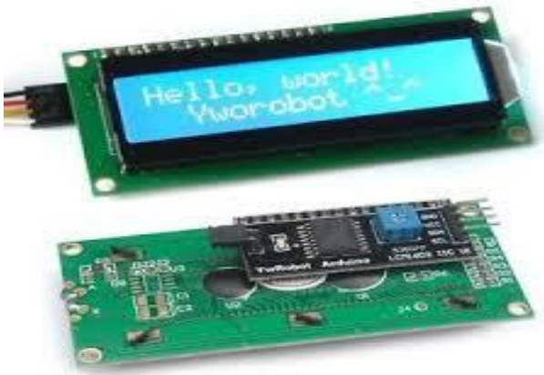
Fig. 5 LCD Display with I2c
