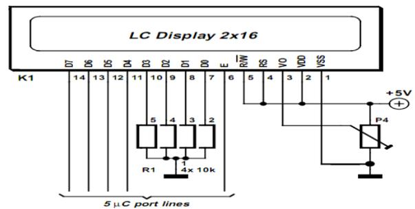
Fig.5 LCD Module Block Diagram
