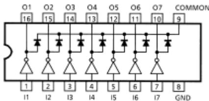
Fig.3 ULN2003A Internal Schematic
