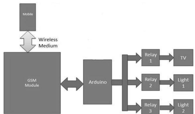
Fig.6 Block diagram of Automation System
