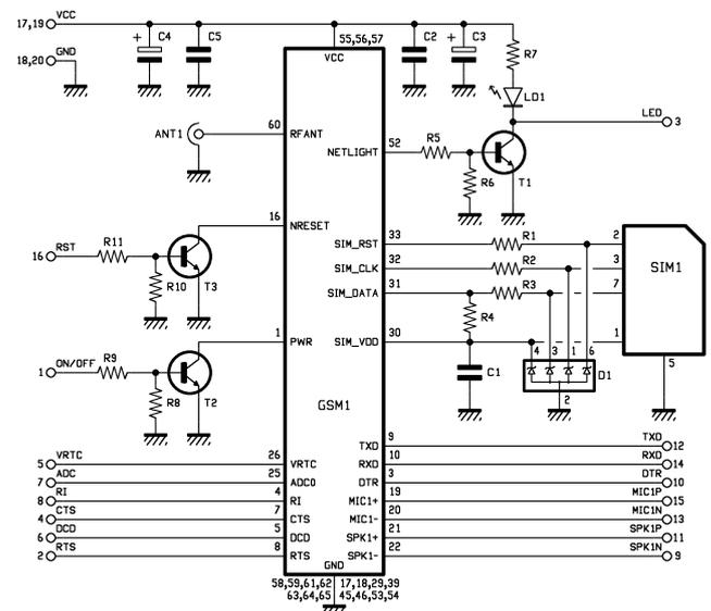
Fig.1 Architecture of GSM900A Module
