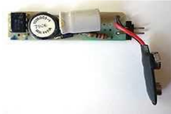
Figure (5): The above DC booster is to boost 2.4V to 9V
