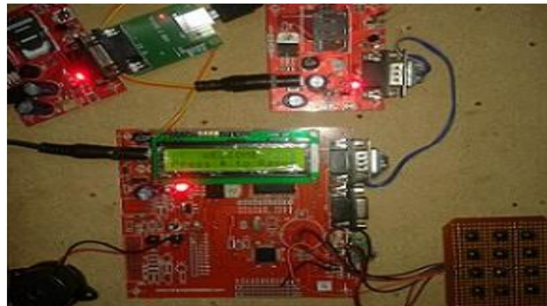
Fig. (d) illustrates a prototype layout of the system when power is on, communication between ARM 7 and GSM at the remote reservation system section.
