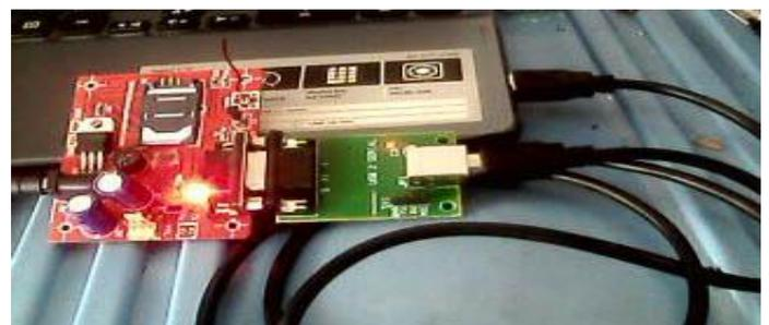
Fig. (e) At the server section communication between the PC and another GSM module
