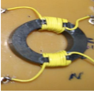
Figure 4.1 Hardware design of CMC
