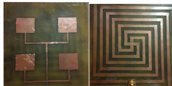
Fig. 8. Practically designed 2X2 array with conventional ground plane
