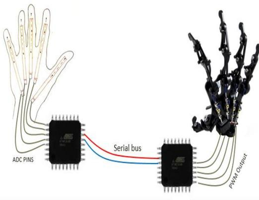
Figure 2.1 Shows configuration of Mechanical Hand and Human Hand
