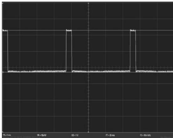
Figure 4.2 PWM output of servo driver on DSO
