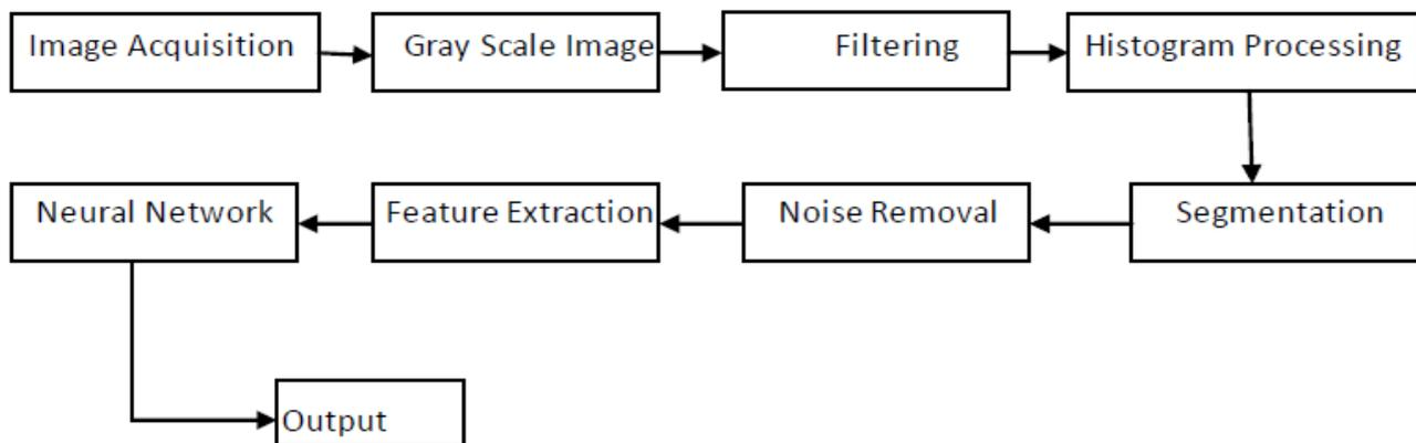
Fig 1: Functional block diagram of proposed system for fabric inspection system
