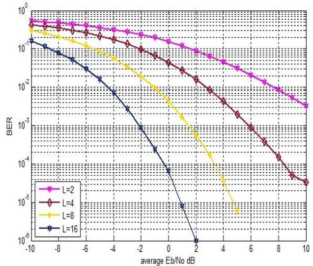
**Figure 3:- BER plot for QPSK for different value of L with  $q=0.5$  and  $\Omega=1$**
