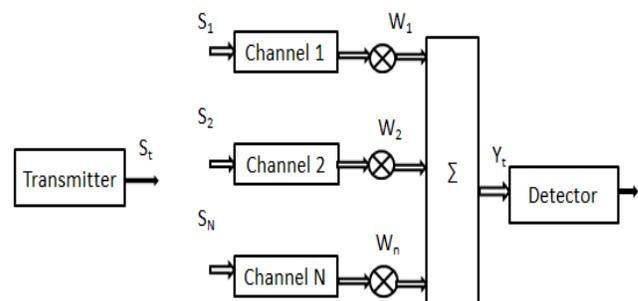
Figure 1-System with MRC Reception
