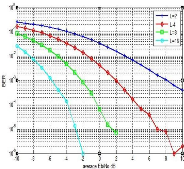
**Figure:-2 BER plot for BPSK for different value of L with  $q=0.5$  and  $\Omega = 1$**
