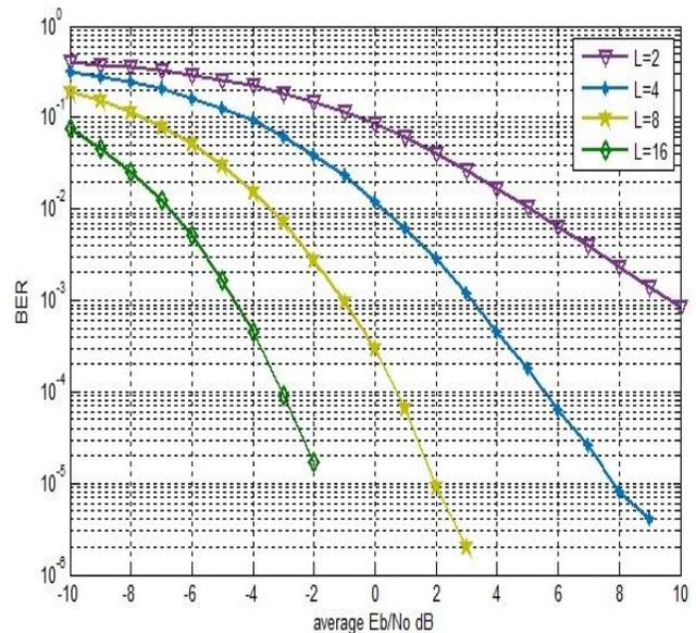
**Figure 4:-BER plot for DBPSK for different value for L with  $q = 0.5$  and  $\Omega=1$**
