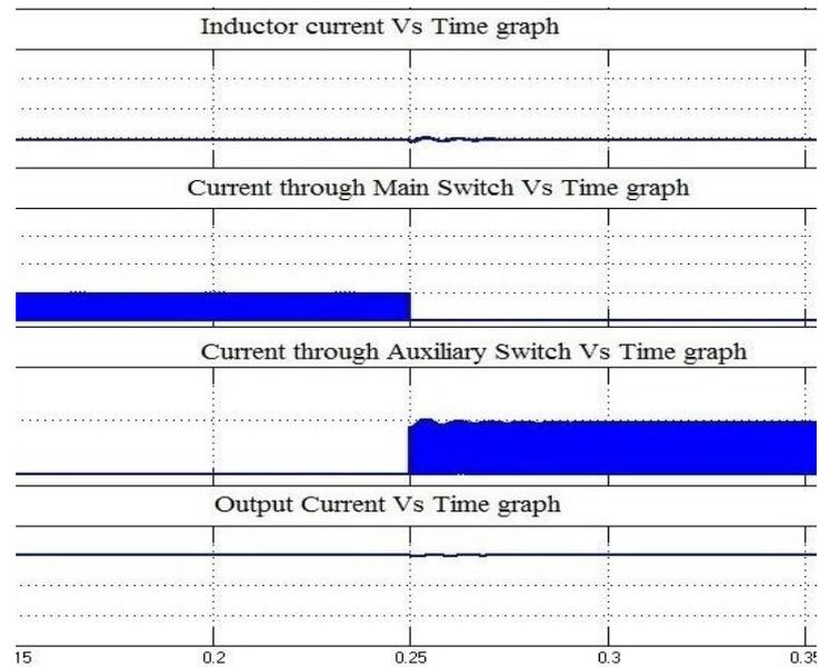
Fig. 7.Open Circuit Fault Rectification
