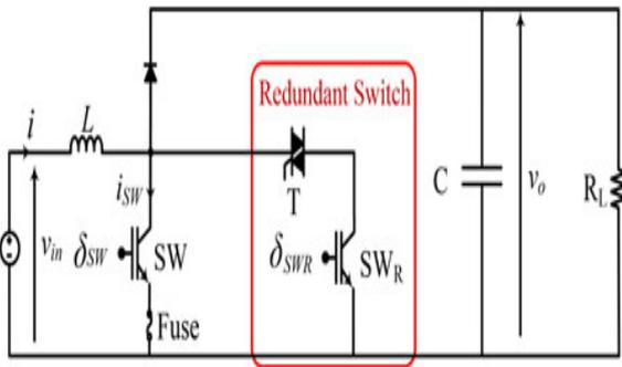
Fig. 1. Boost converter incorporating fault tolerant operation
