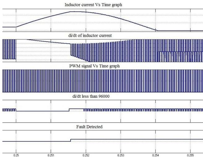
Fig. 9.Short Circuit Fault Detection
