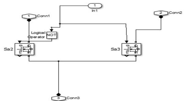
Fig. 4. Boost Converter-Sub System
