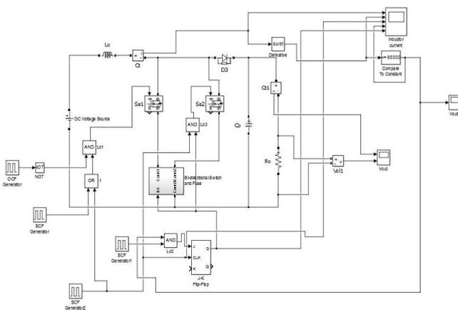
Fig. 2. Boost Converter Open Circuit
