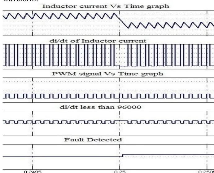
Fig. 6.Open Circuit Fault Detection
