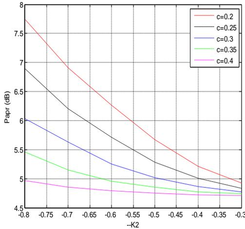
fig.2 (a) the ultimate PAPR of the companded signal
