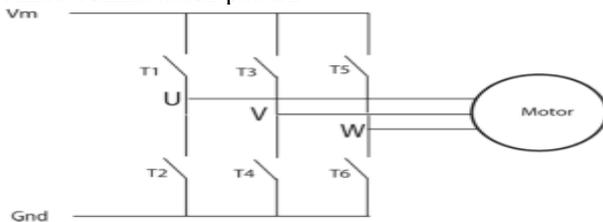
Fig.3. The three half bridges have six power switches.
