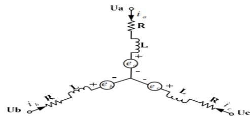
Fig. 4. Equivalent circuit model of BLDC
