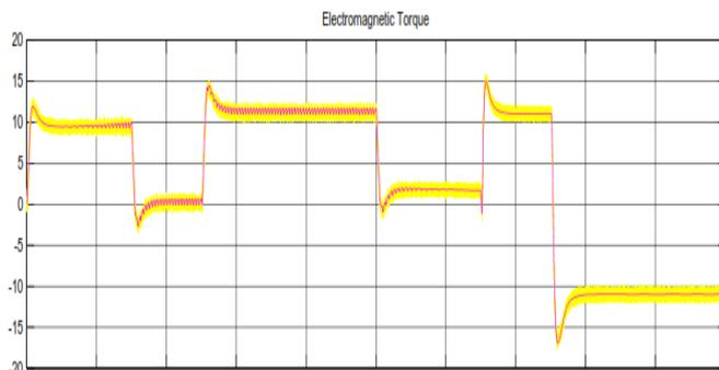
Fig.7. Electromagnetic Torque of BLDC motor.
