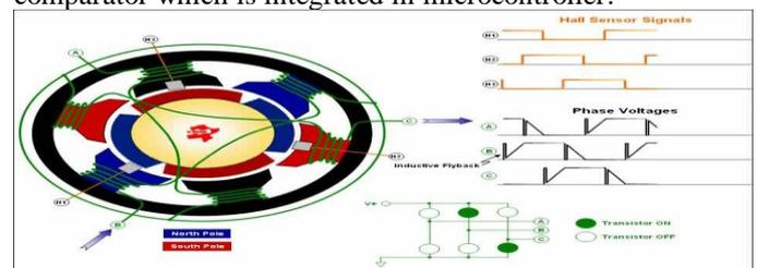
Fig.2. Brushless DC Motor With Hall sensor & Phase Voltage.
