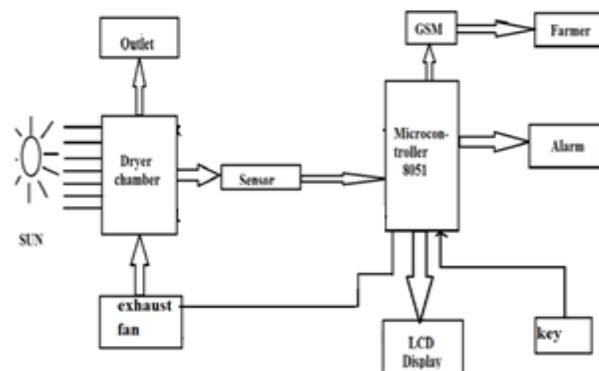
Fig 1:-Block diagram of fruit drying system
