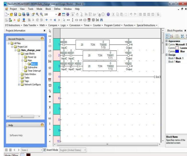
Figure 4: Ladder diagram programming used in PLC
