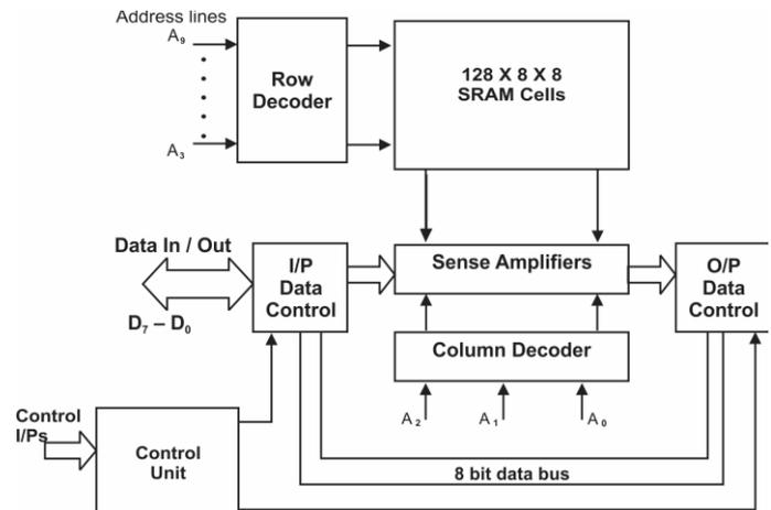
**Figure 1:** Block Diagram of 128x128 SRAM Cells.
