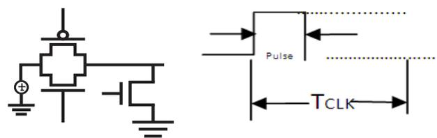
Figure 4: Pulse Circuit with pulse output.
