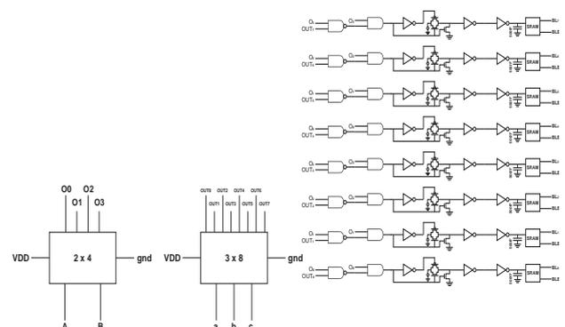
Figure 5: Block Diagram of Complete Pulse Decoder Circuit
