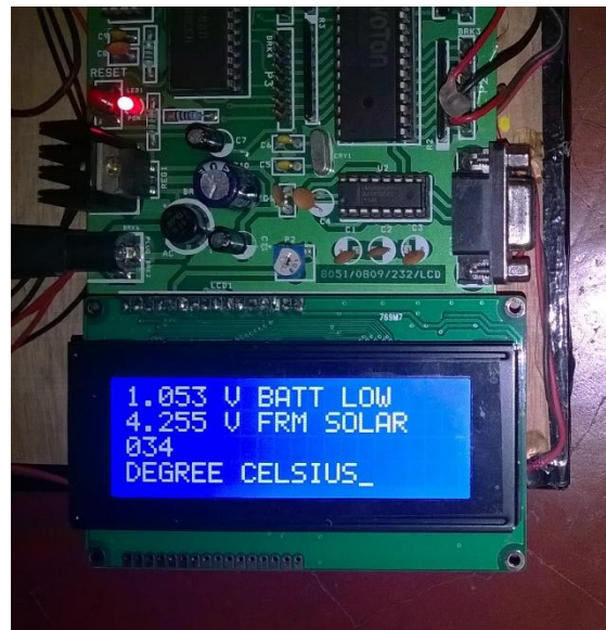
Fig (h): Display of battery level and temperature value on LCD.
