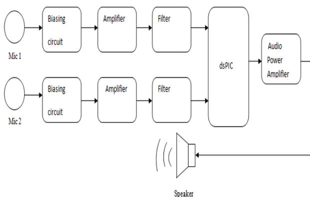
Fig. 3.1 Block diagram of noise suppressor
