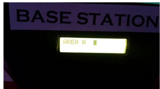
Fig 10: Crash location display at the base station
