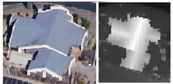
Fig. 2. Second example: Digital map of the area where Lidar is collected and the generated DSM model
