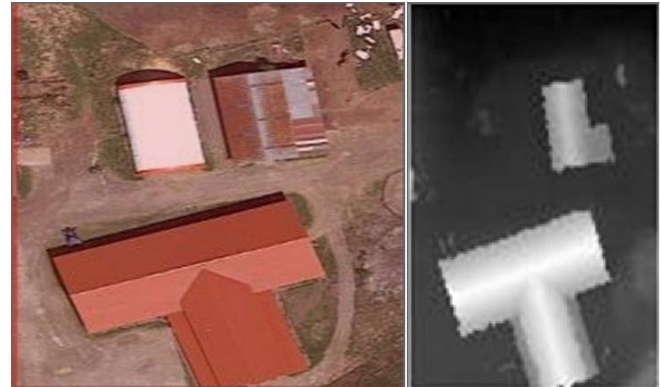
Fig. 1. Digital map of the area where Lidar is collected and the generated DSM model
