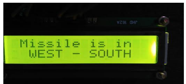
Figure 12: The output on LCD when the missile is detected in West-South direction.
