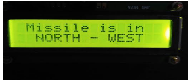
Figure 10: The output on LCD when the missile is detected in North-West direction.
