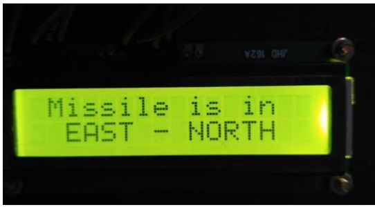
Figure 13: The output on LCD when the missile is detected in East-North direction.
