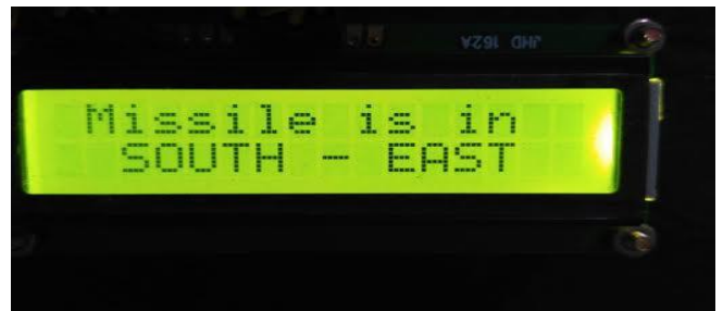
Figure 11: The output on LCD when the missile is detected in South-East direction.
