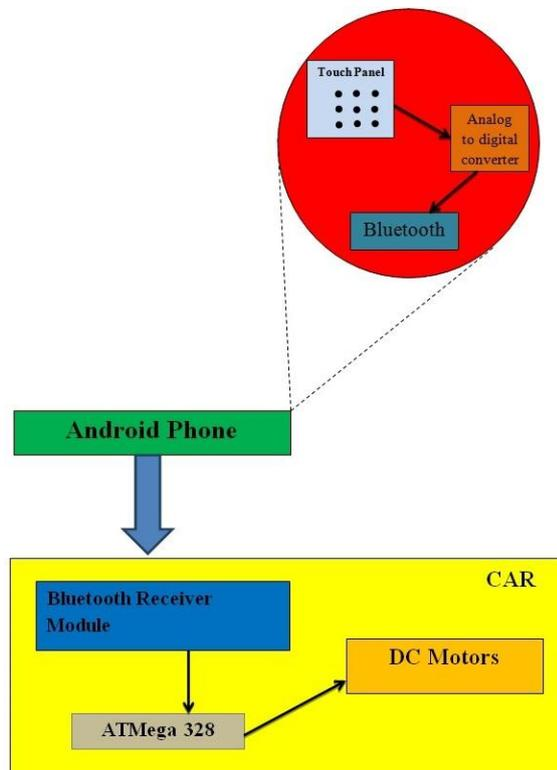
**Figure 1: Block Diagram**
