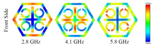
Fig. 8. Electric field distributions at the resonant frequencies of one cell for microwave frequency region.
