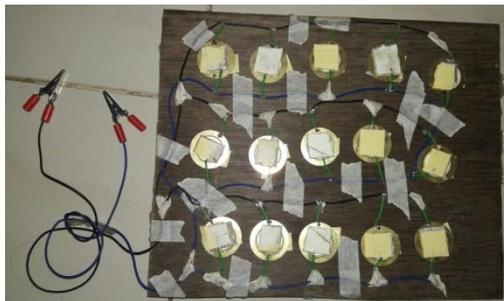
Fig 2: connection of piezoelectric sensor
