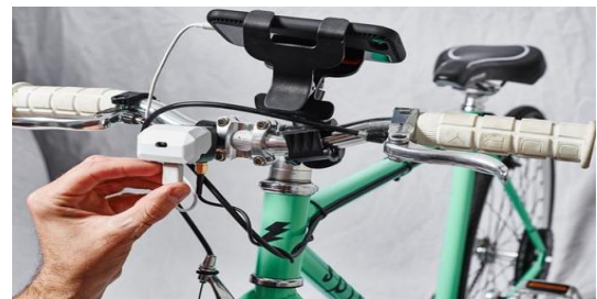
Fig.1.1 Bicycle with Smartphone and charging assembly
