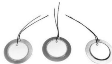
Figure2. Piezoelectric discs used
