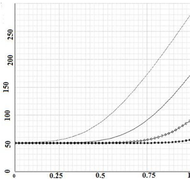
Fig 5: FGMOS Transfer Characteristics
