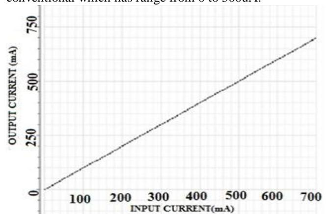
Fig 7: Input current vs Output current characteristics of proposed current mirror
