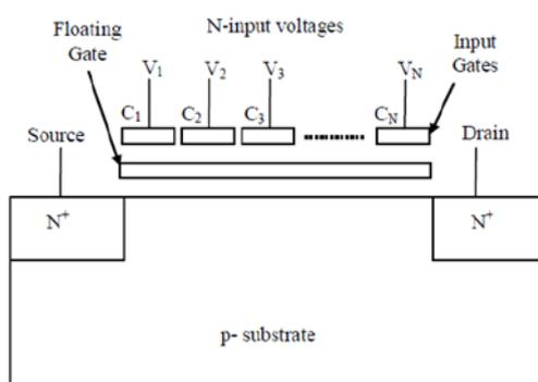
Fig 2: Structure of Floating gate MOSFET.
