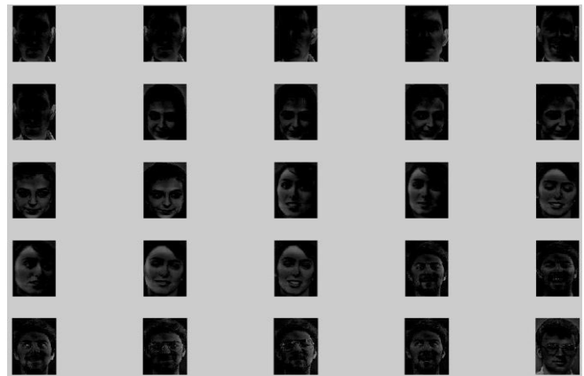
Figure 6.3: Represents some examples of eigenfaces [12].
