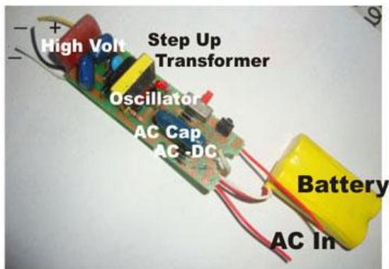
Fig (c): Shockwave generator
