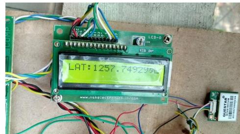
Fig (e): The GPS location of the victim's latitude and longitude will be sent to the Police Station.
