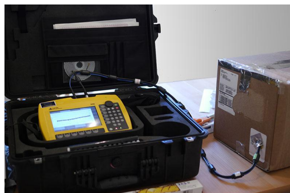
Fig.4) Test Setup for SRM-3006 Meter
