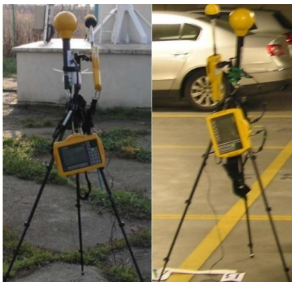
Fig.5) SRM Meter Setup in Work Place
