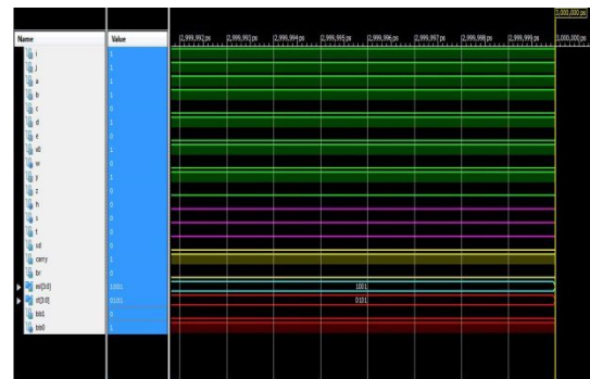
Fig.9 simulation result of proposed ALU
