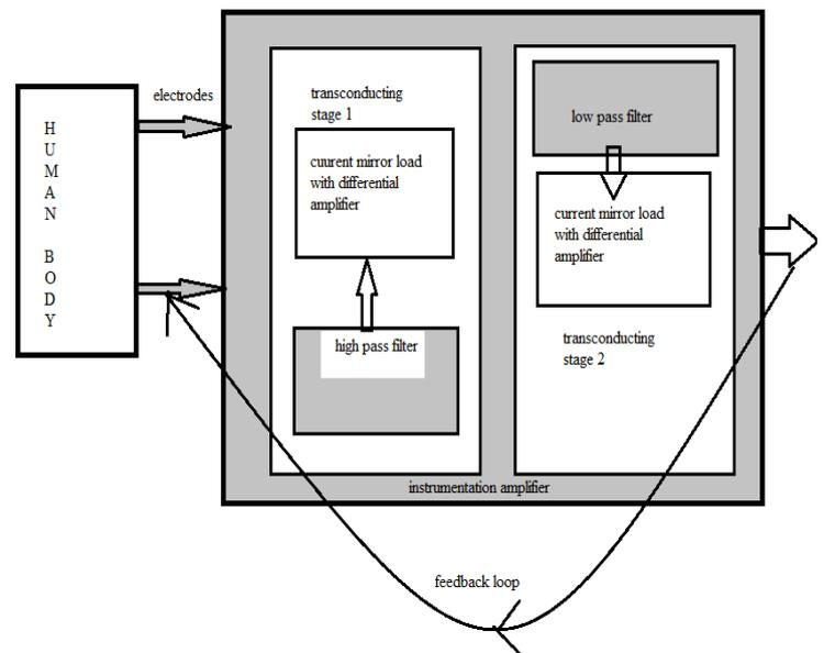
Fig. 1 Block diagram of proposed instrumentation amplifier.
