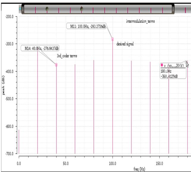
Fig.6 intermodulation terms of the simulated filter.
