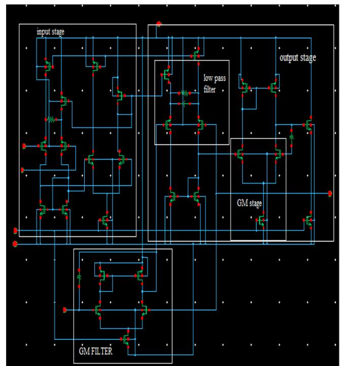
Fig. 2 schematic diagram of proposed IA
