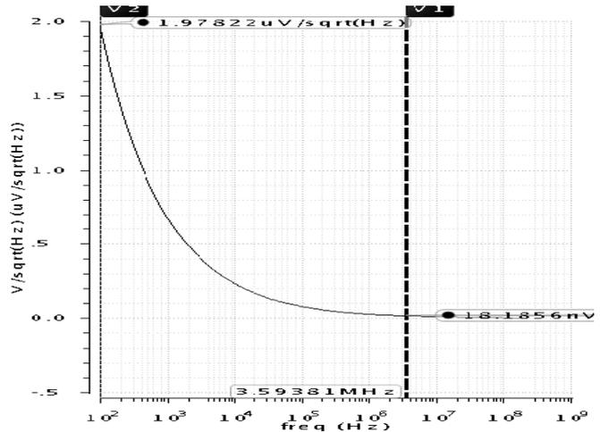
Fig. 7 input referred noise of the filter
