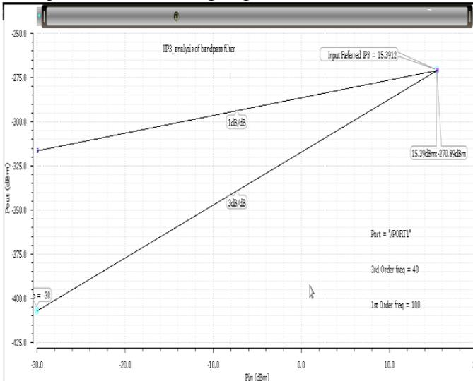
Fig. 5 IIP3 analyses of bandpass filter in IA.
