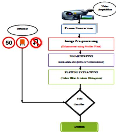
Figure 4.1: Process flowchart
