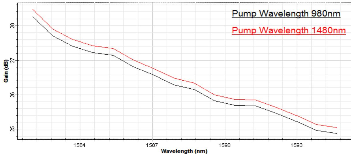
**Figure 5 :Gain curve for pump wavelengths**
