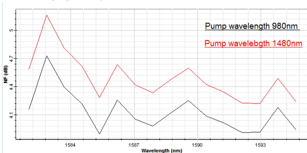
**Figure 6 :Noise Figure curve for pump wavelengths**
