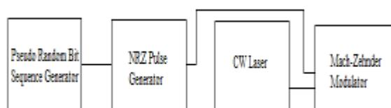
**Figure 2: Block Diagram of Transmitter**
