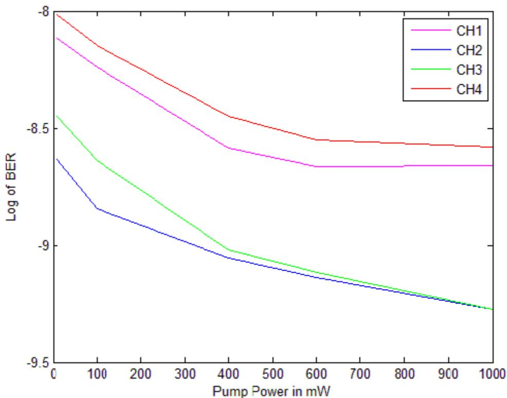
**Figure 4: pump power versus BER**
