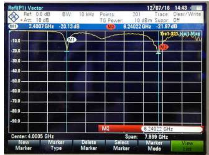
Figure 14: Measured Return loss ( S_{11} ) using VNA
