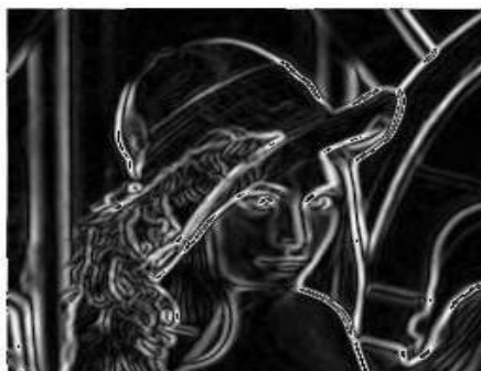
Figure 5: The edge detection using Sobel detector
