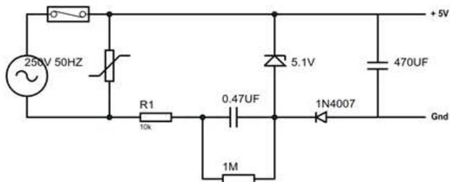
Fig. 9 Circuit diagram of dc 5volts regulated power supply
