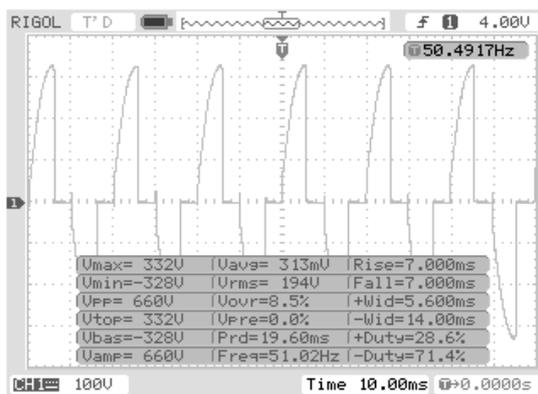
Fig. 17 waveform across triac output at speed level five (194 Volts)
