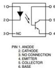
Fig. 7 pin diagram of MCT2
