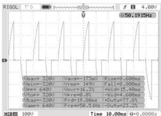
Fig. 15 waveform across triac output at speed level three (149 Volts)
