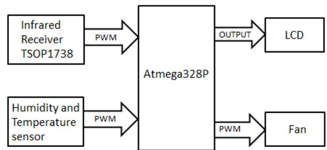
Fig. 1 Block diagram of fan speed control system
