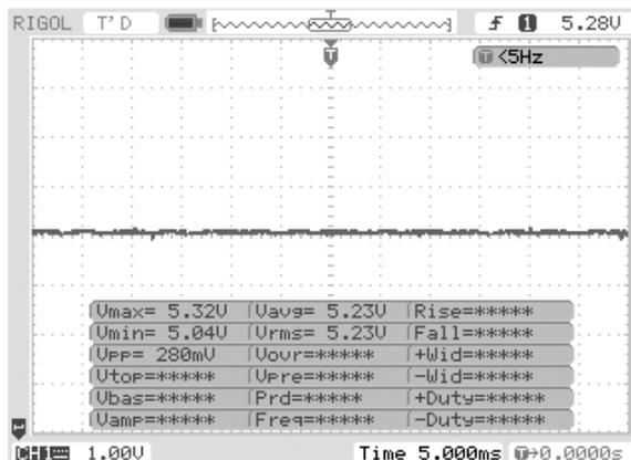
Fig. 18 waveform across dc 5volts power supply
