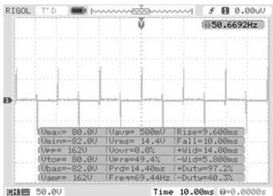
Fig. 13 waveform across triac output at speed level one (14.4 Volts)
