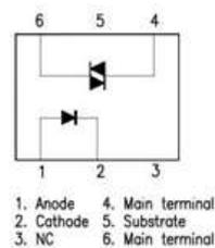
Fig. 6 pin diagram of MOC3021
