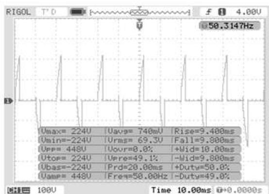
Fig. 14 waveform across triac output at speed level two (69.3 Volts)
