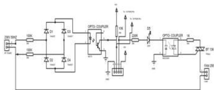
Fig. 10 Zero Crossing Circuit
