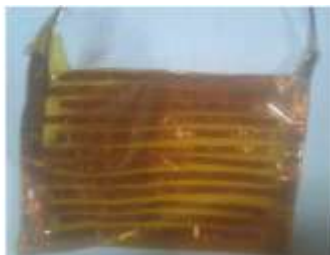
Fig. 2. Prototype of electroadhesive pad using polyimide film.
