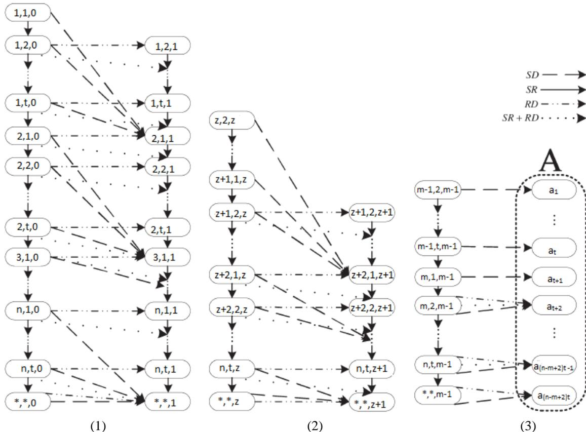
Fig.3. absorbing Markov chain for 2HR-( $m, n, t$ ) algorithm.
