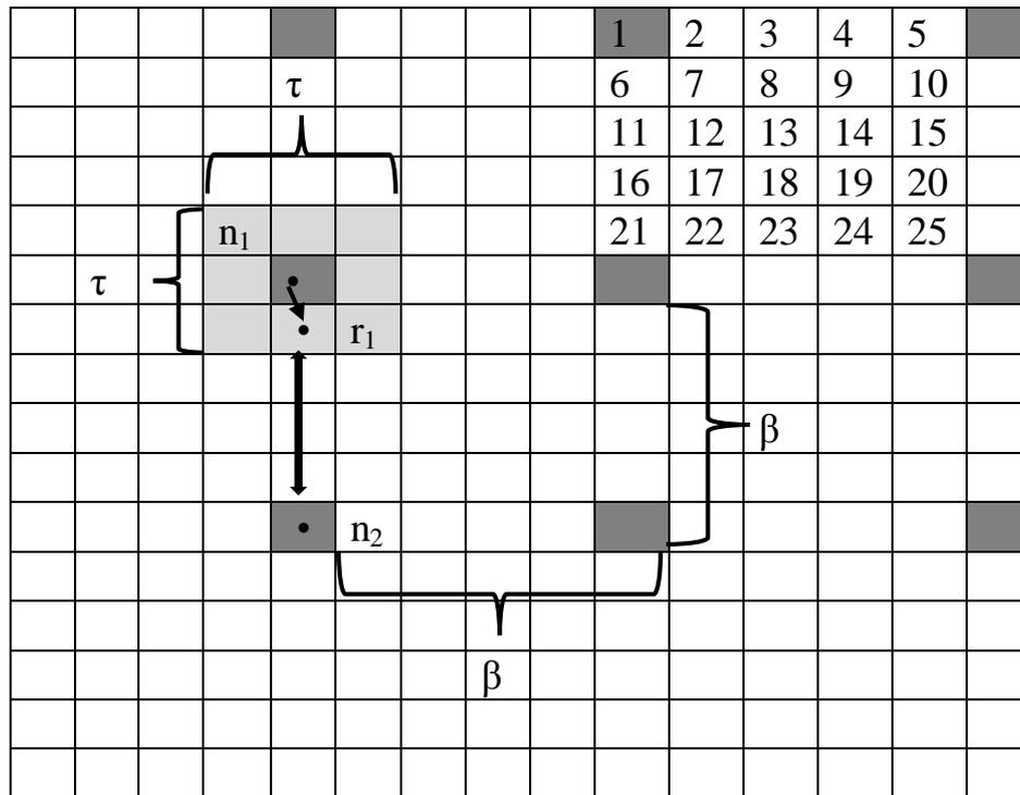
Fig.1. network model and an example of transmission scheduling with the case  $x=15$ ,  $\tau=2$ , and  $\beta=5$ .
