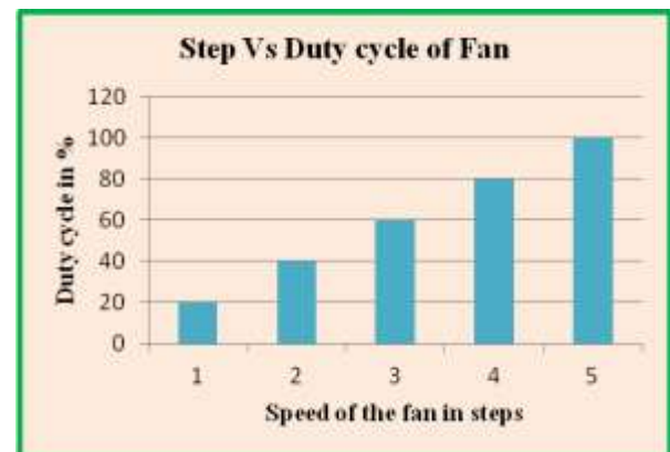
Figure 8. Step Vs Duty cycle of Fan
