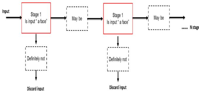
The overall process of face detection is described in below picture
