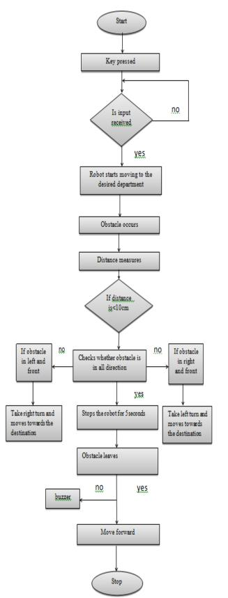
Our robot is placed at entrance default and if the entrance key itself is pressed the robot doesn't move. If some other department key is pressed the robot moves towards the department, on the way if any obstacle is detected in all direction the robot stops for some second still obstacle doesn't move in any direction buzzer starts ringing, if any one direction is free robot takes that direction without deviating it reaches the location.
