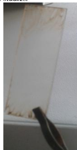
Fig. 3. ZnO thin film deposited on glass substrate
