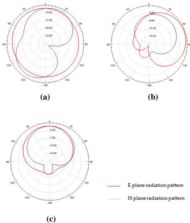
Figure 5 Radiation pattern (a) Azimuth and elevation plane at 2.7 GHz (b) Azimuth and elevation plane at 5.1GHz (c) Azimuth and elevation plane at 7.2GHz
