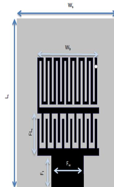
Figure 6 Design of antenna with inter digital capacitor and grounded meander line-II ( $L_s=10\text{mm}$ ,  $W_s=10\text{mm}$ ,  $W_b=7\text{mm}$ ,  $F_w=3\text{mm}$ ,  $F_l=2.5\text{mm}$ ,  $F_{Lc}=3\text{mm}$ ).
