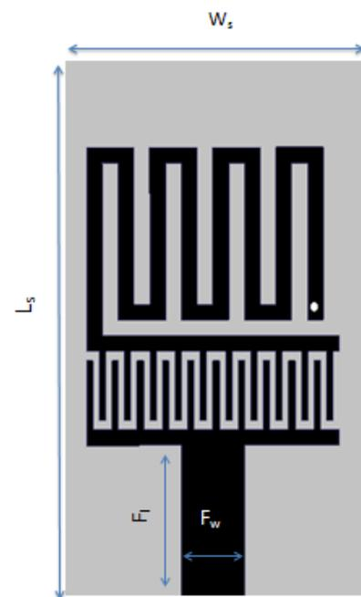
**Figure 2 Layout of antenna with inter digital capacitor and grounded meander line-I ( $L_s=18\text{mm}$ ,  $W_s=10\text{mm}$ ,  $W_b=7\text{mm}$ ,  $F_w=2\text{mm}$ ,  $F_l=5\text{mm}$ ).**
