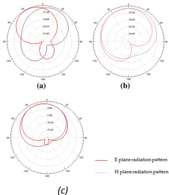
Figure 9 Radiation pattern (a) Azimuth and elevation plane at 1.1 GHz (b) Azimuth and elevation plane at 3.7GHz (c) Azimuth and elevation plane at 6.8GHz
