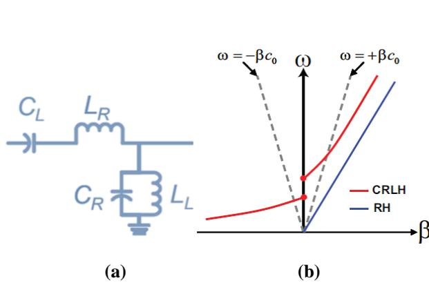
**Figure 1 CRLH TL unit cell (a) Equivalent circuit model (b) Dispersion diagram**
