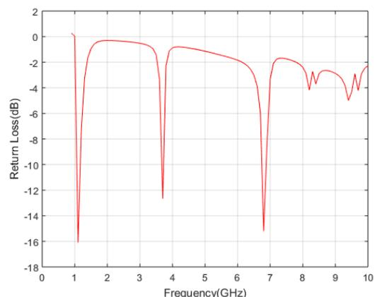
Figure 7 Simulated Return Loss
