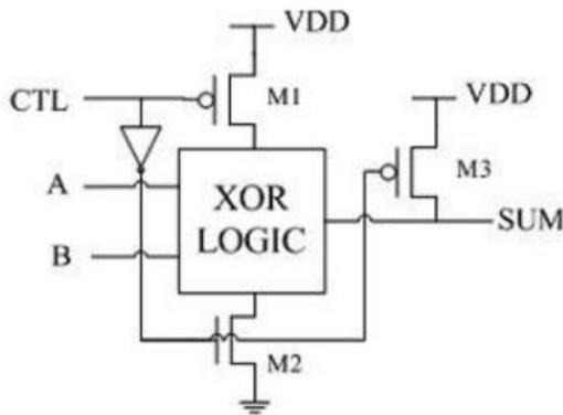
Fig: 7 design of modified XOR block
