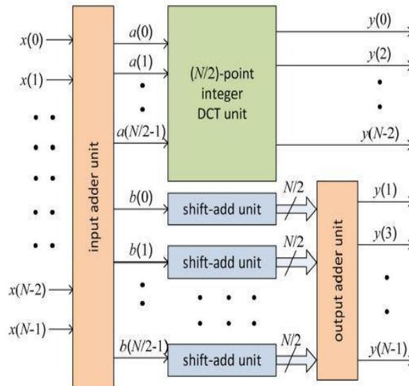
Fig.2 reusable DCT architecture for N = 4,8,16 and 32
