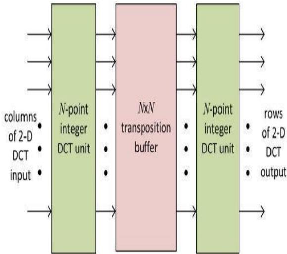
Fig. 3 Full parallel 2D DCT architecture
