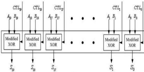
Fig: 6 design of carry-free addition block
